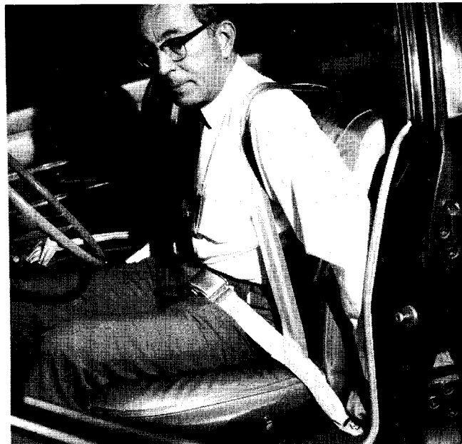
C Shoulder belts slipped on like suspenders and only lap belt buckle to fasten.
