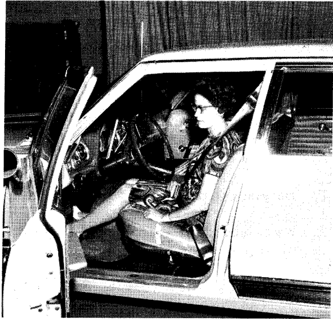
B Subject dons restraint equipment by grasping tongue of buckle with right hand and pulling over left arm and shoulder.
