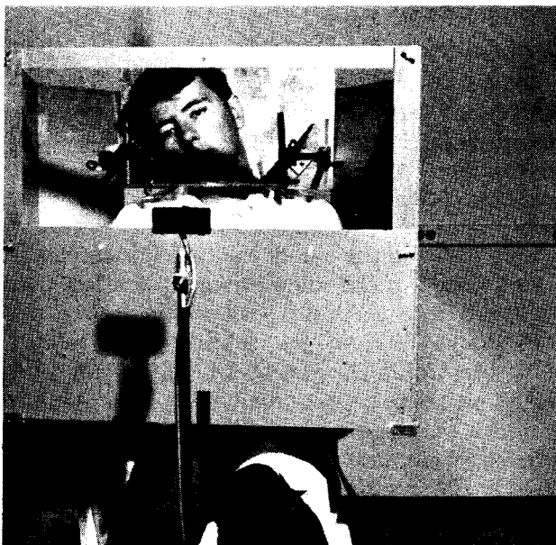
FIGURE 1. Several views of the stimulator. Upper left: experimental arrangement for the total darkness and the wing-tip lights conditions. Upper right: the cabin frame (minus the front panel) has been added. Lower left: front panel added to cabin frame with the subject's head in the right tilt position. Lower right: interior view of the cabin frame condition (wing-tip lights were viewed through the "window" of the cabin).
