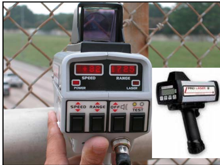
Figure 27. Speed Data Collection Using Lidar (Radar) Gun.
