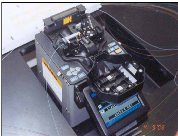
Figure 8-3: Fusion Splicing Fiber Strands - Photograph Courtesy Adesta, LLC
