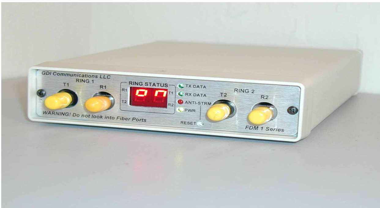
Figure 6-1: Photograph of a Fiber Optic Modem - Courtesy GDI Communications, LLC
