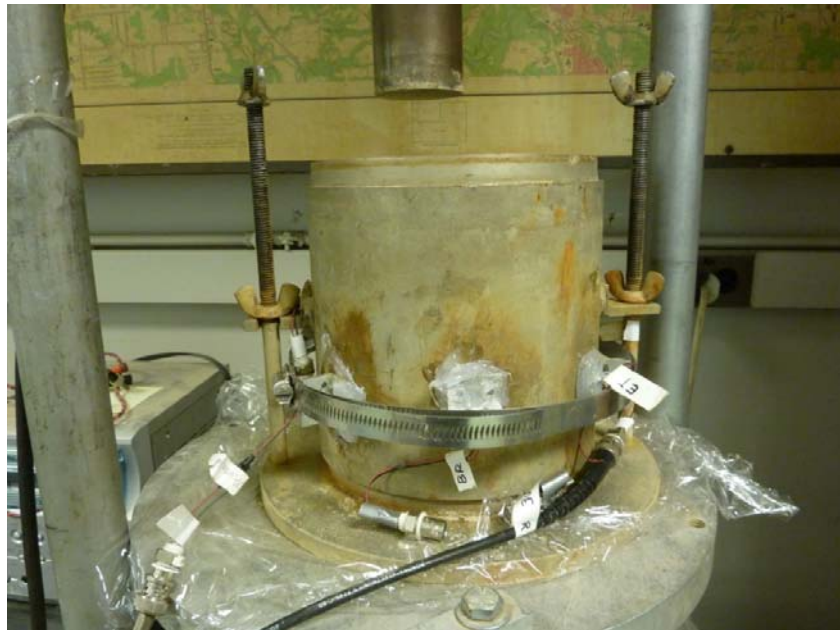
Fig.4 Bender and Extender Element Test Set-up
