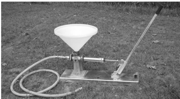
Figure 2.10. CG-050M manual grout pump.
