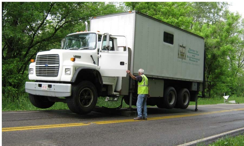
Figure 2.5. Heavy-duty CPT truck in level condition.
