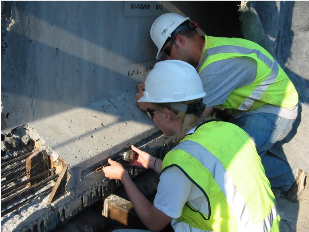
Figure D-4: Researchers Jennifer Dunbeck and Brett Holland taking DEMEC readings.
