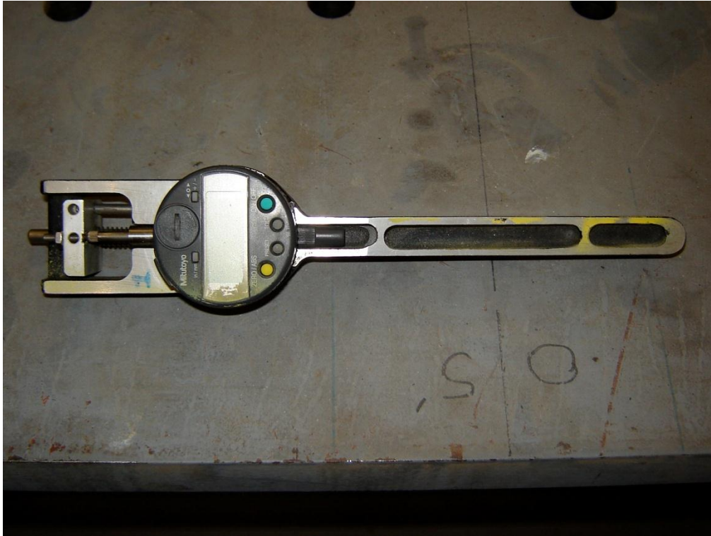
Figure D-3: DEMEC gage used for this research.
