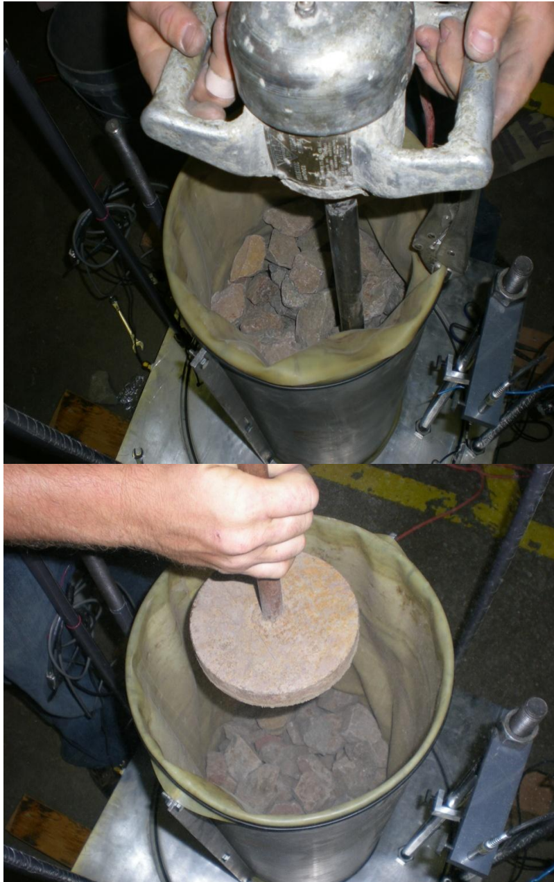
Figure 3.6 Proposed Compaction Process: Rearranging Particles with Vibratory Rod (Left) and 45-N Dropping Plate for Densification (Right)
