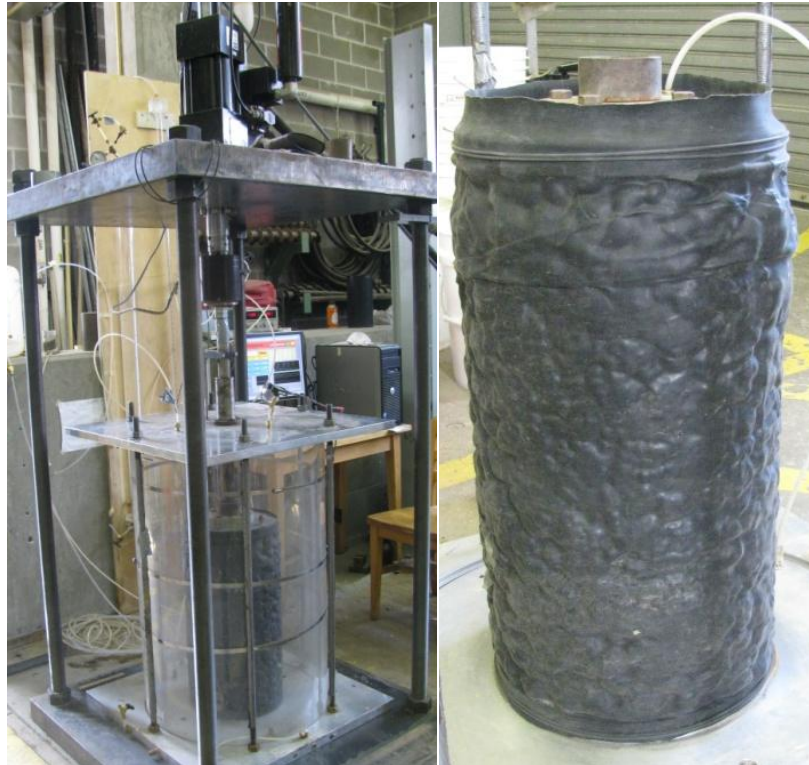
Figure 4.3 Large-Scale Cyclic Triaxial (LSCT) Apparatus for Ballast Testing (left) and a Prepared Railway Ballast Specimen before Testing (right)
