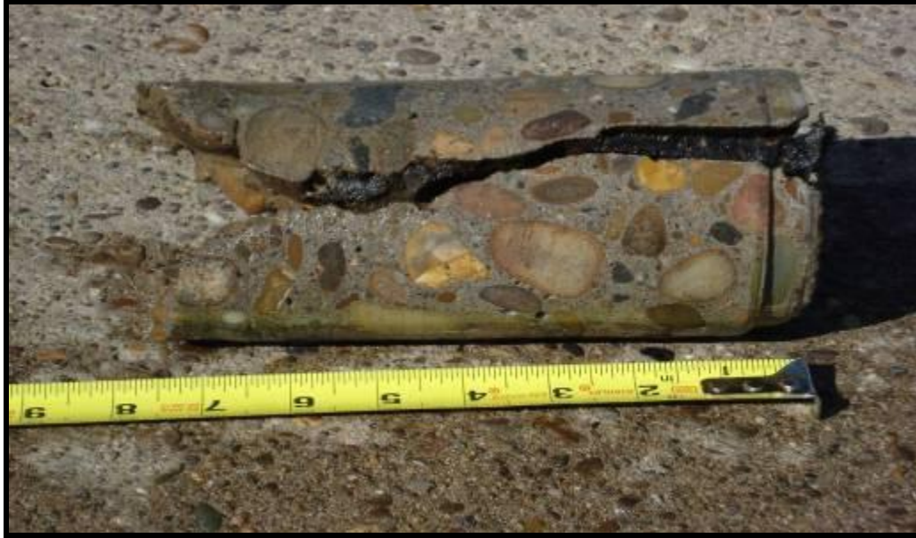
Figure F23. – Side of Core at Joint
