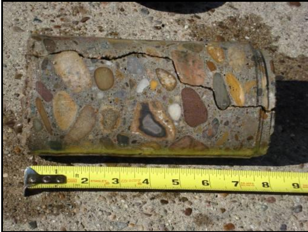
Figure F21. – Transverse Crack through Core
