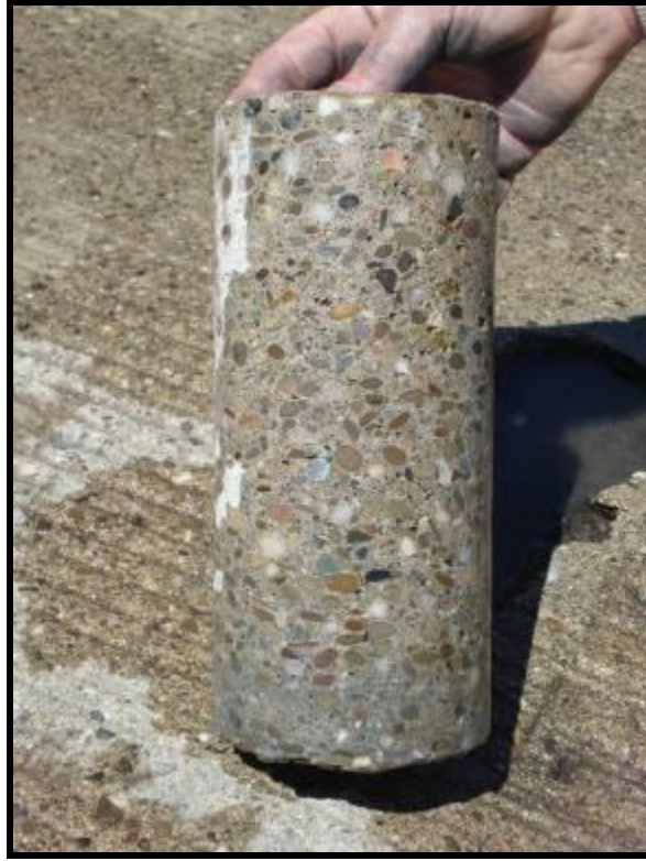
Figure F10. - #8 Gravel Aggregate in Midslab Core
