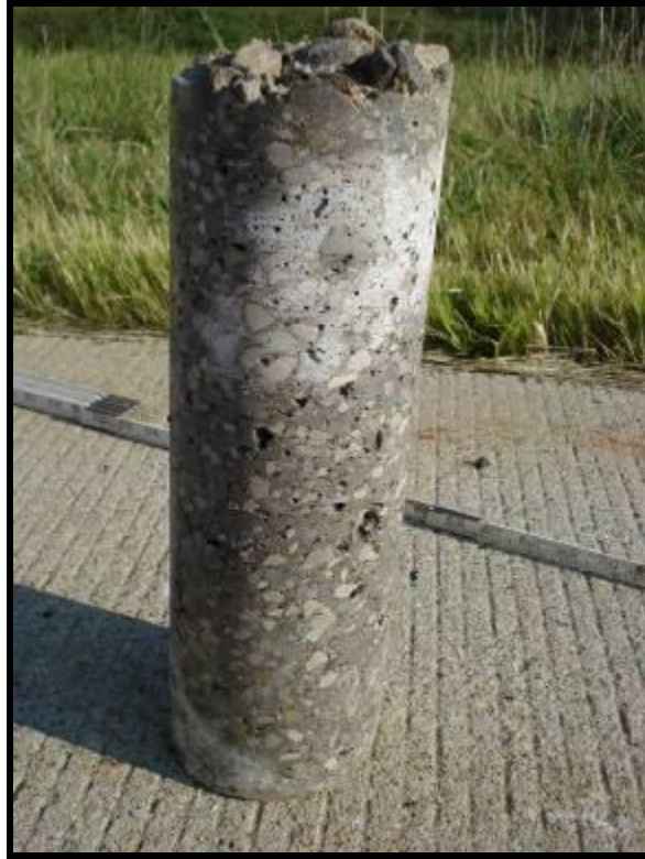
Figure F31. – Voids in Core
