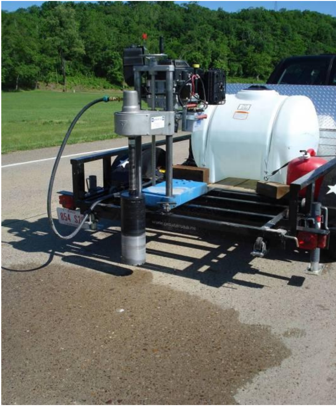
Figure 3.2 – Core Rig Fabricated by ORITE
