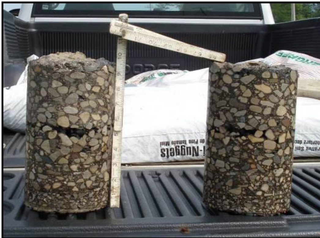
Figure E7. – Voids in 301 AC Base
