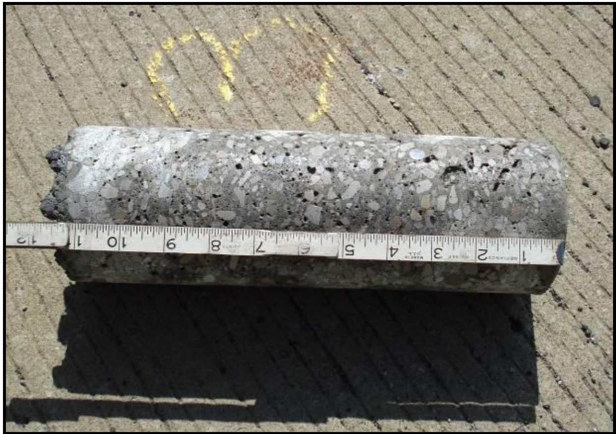
Figure F19. – Air Voids in CUY 176 12 S Core
