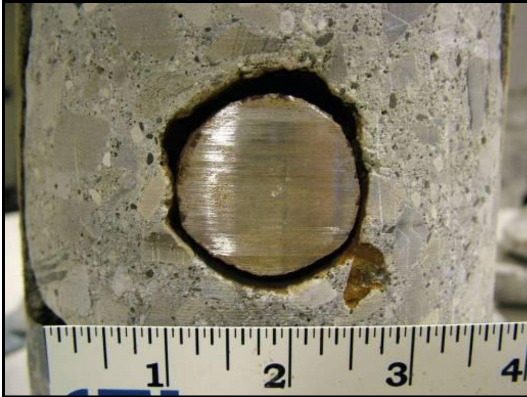
Figure F4. – Void around Dowel Bar at Construction Joint
