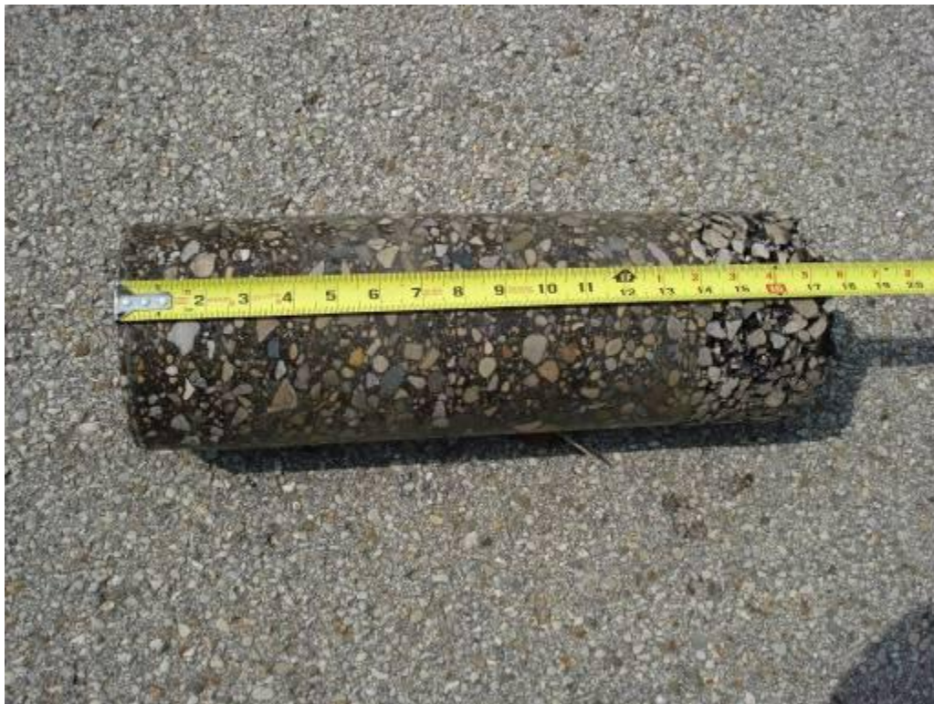
Figure E25. – Intact Core Showing Material Layers
