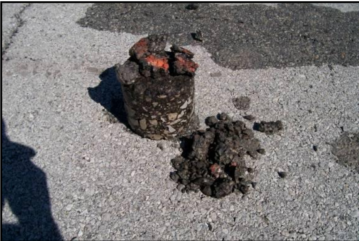
Figure E12. – Delamination of Core in Section 112 on DEL 23
