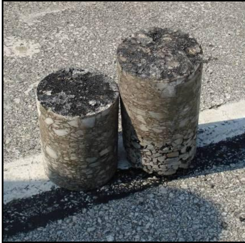
Figure E3. – Delaminated 302 over ATFD Base
