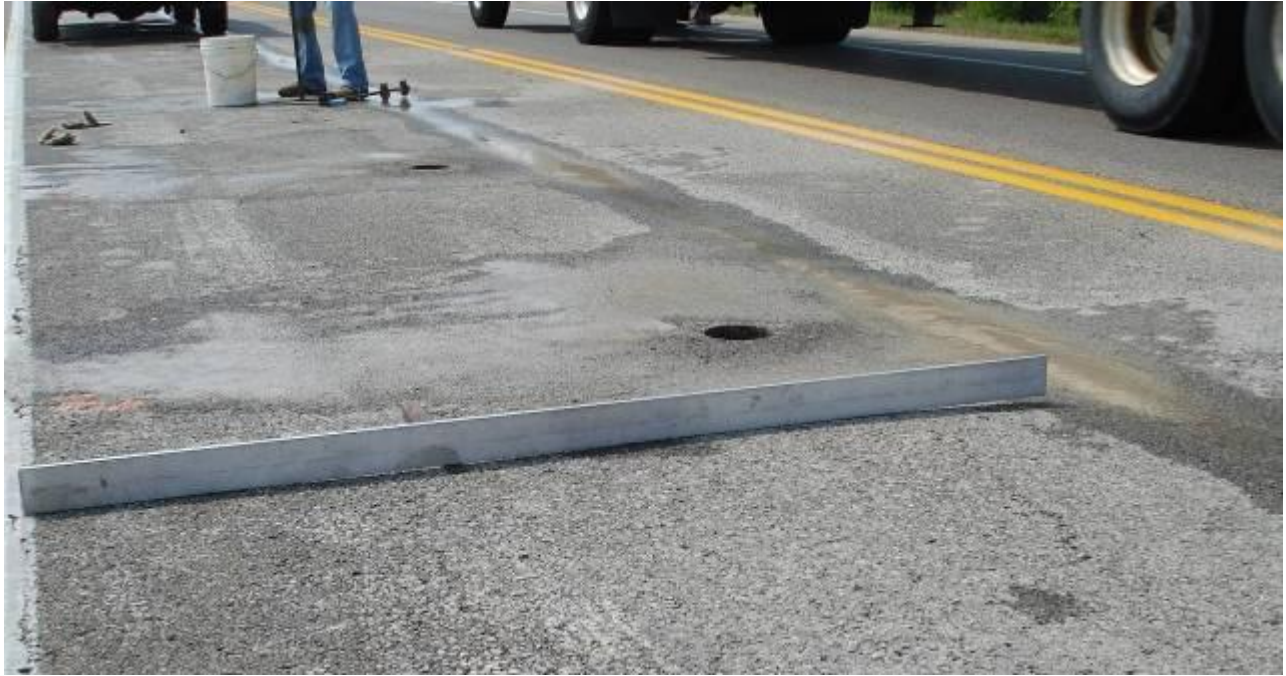
Figure E6. – Rutting in CHP 68 2.5N
