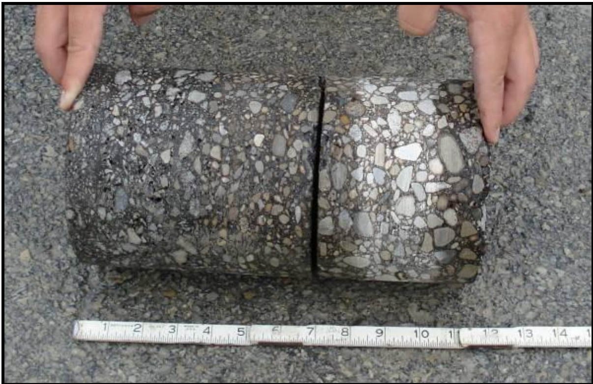
Figure E14. – Delamination of 301 on GRE 35 21E
