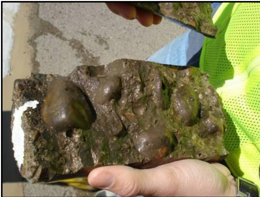
Figure F22. – Fracture Plane in Core
