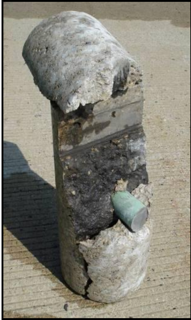
Figure F18. – Horizontal Cracking at Dowel Bars
