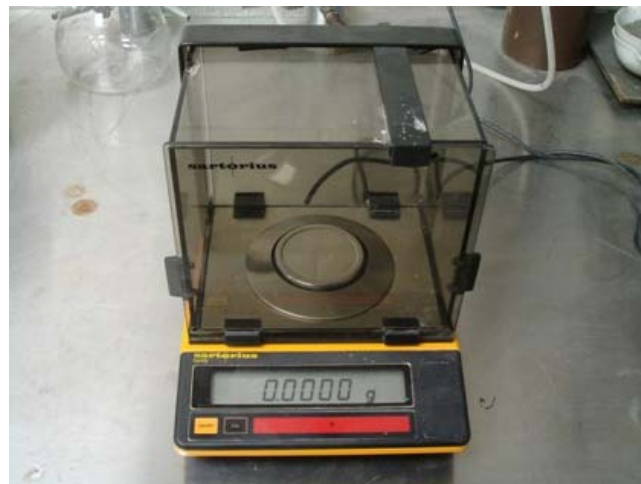
Figure 3.15. Weighing Balance Used in Measuring the Weight of the Filter Papers.
