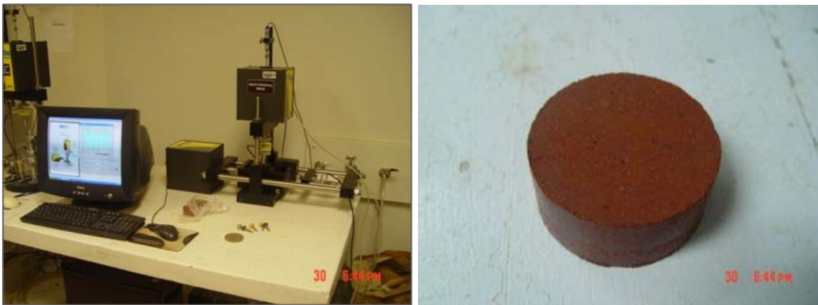
Figure 3.24. The Direct Shear Test Setup and Compacted Silty Sand Used in the Test.
