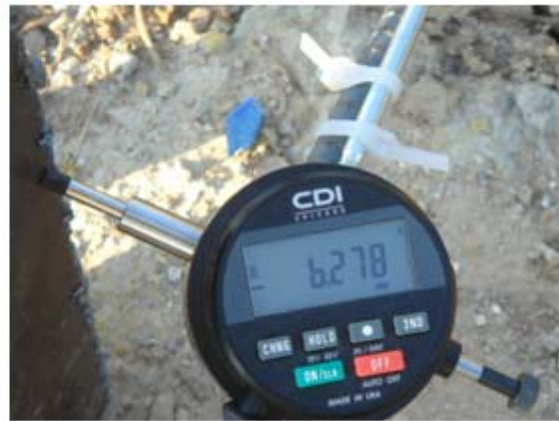
(b) Test Shaft Deflection Due to Loading
