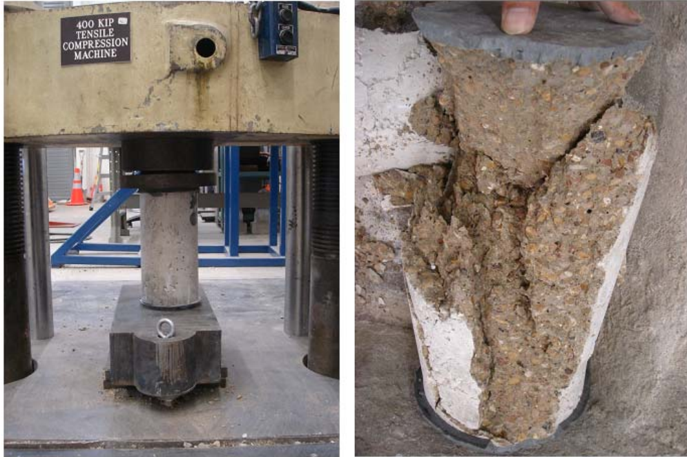
Figure 4.19. Compressive Strength Test Setup and Failed Concrete Specimen.
