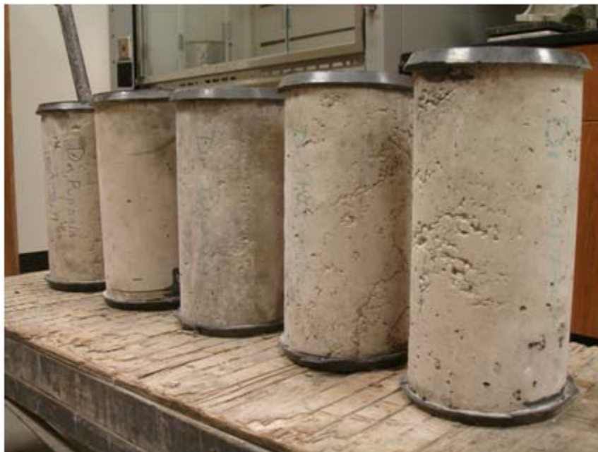
Figure 4.17. Concrete Cylinder Specimens with Capping Compound.
