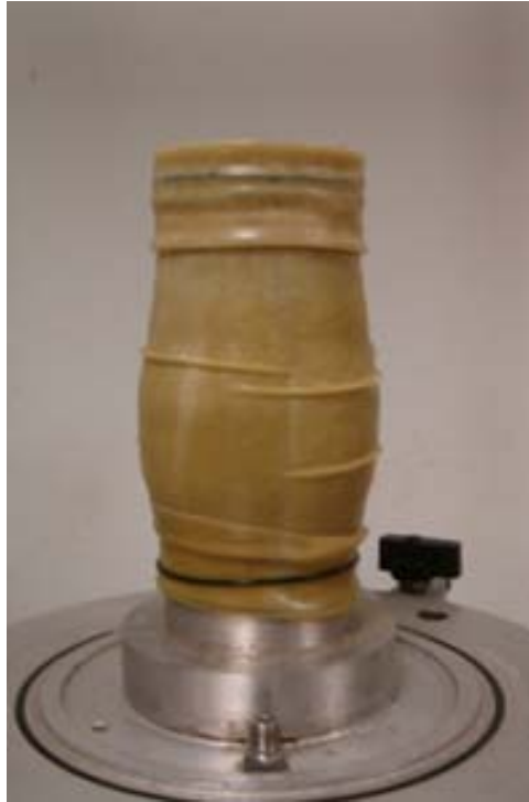
Figure 3.27. The Failed Specimen Performed by Triaxial Test.
