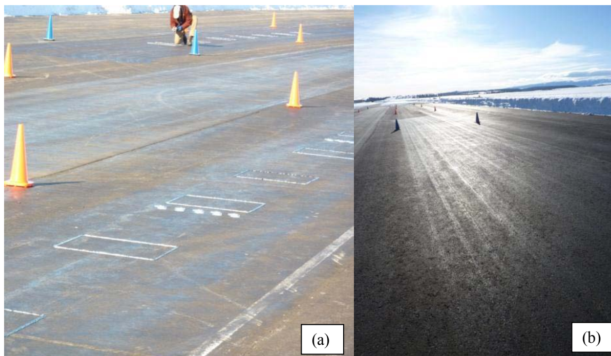
Figure 22 Petri-dish set placement near sample plot prior to application of the anti-icer NaCl+GLT (a) and drill mark patterns of the anti-icer FreezGard obvious in the sunlight (b).
