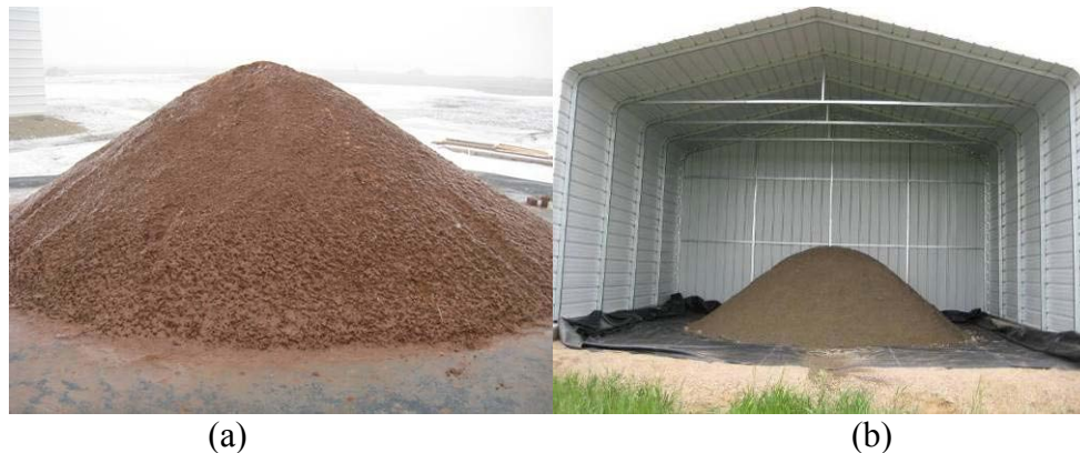
FIGURE 2 Photograph of (a) uncovered IceSlicer on the outdoor slope pad and (b) a 10% salt-sand mixture inside the storage facility at TRANSEND.
