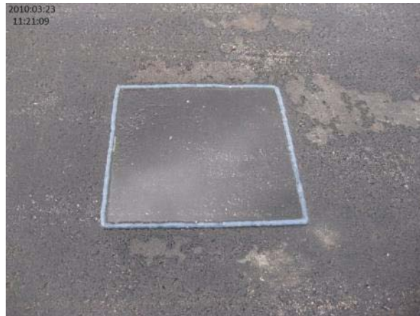
Figure 32 Sample test box containing free standing water in the day 4 FreezGard test lane.
