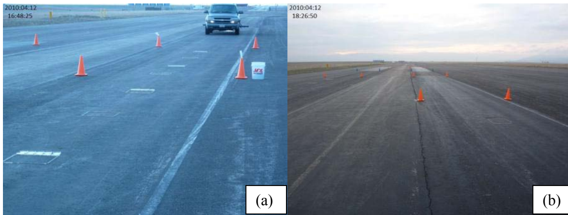
Figure 34 Clearing and washing chosen test section within the driving surface area using a plow truck and high pressure hose.
