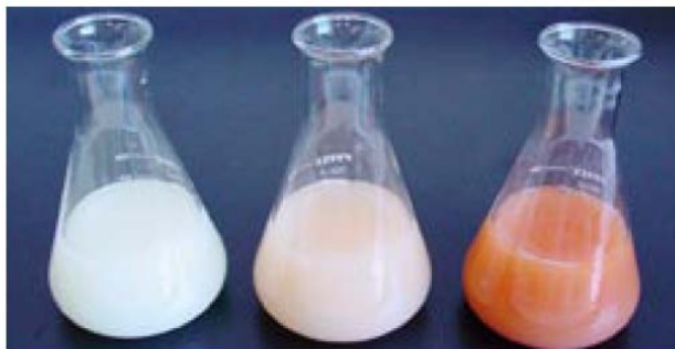
Figure 2 Left flask: before the titration endpoint, addition of \text{Ag}^+ ions leads to formation of silver chloride precipitate, making the solution cloudy. The chromate indicator gives a faint lemon-yellow colour. Centre flask: at the endpoint, all the \text{Cl}^- ions have precipitated. The slightest excess of \text{Ag}^+ precipitates with the chromate indicator giving a slight red-brown colouration. Right flask: If addition of \text{Ag}^+ is continued past the endpoint, further silver chromate precipitate is formed and a stronger red-brown colour results. NB: The titration should be stopped when the first trace of red-brown colour is observed. Using an incompletely titrated reference flask for comparison is a helpful way to identify the first appearance of red-brown colouration.
