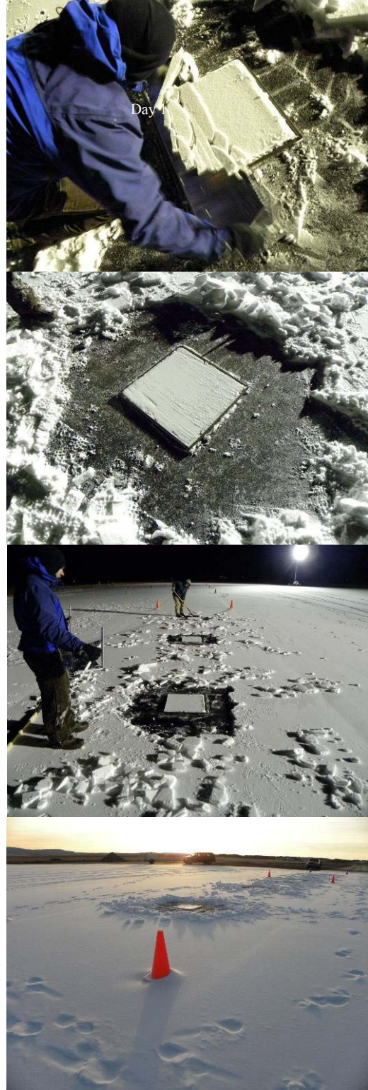
Leveling the snow content in the squares prior to the sample collection
