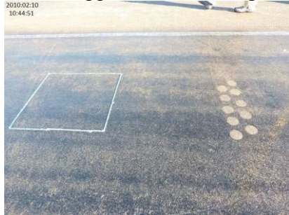
Deicer Application showing Petri dish location
