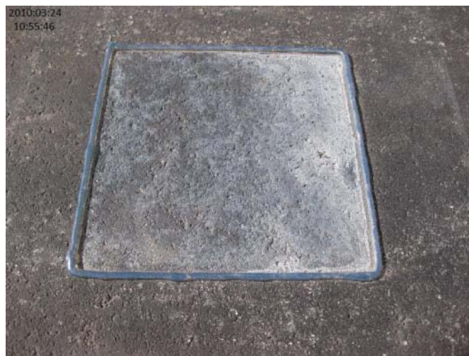
Figure 33 Evidence of the applied liquid deicer NaCl+GLT remains in the test box
