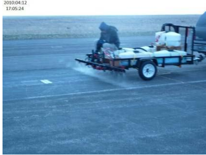
Deicer Application showing Petri dish location
