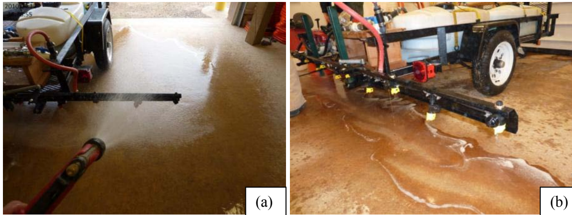
Figure 35 Garden hose with spray nozzle used for rinsing (a) and final flush with the next anti-icer (b).
