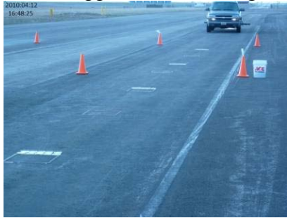
Deicer Application showing Petri dish location
