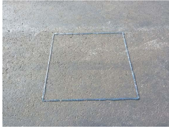
Figure 18 Example of a sample box (18 by 18 inches) laid out on the asphalt surface within a test lane using silicone sealant.
