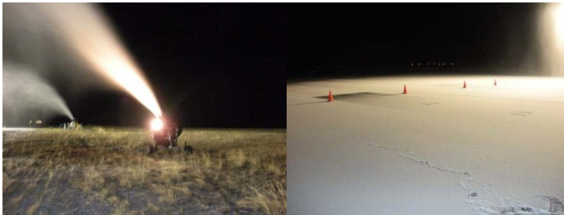
Figure 29 Snow guns making snow over test sections.
