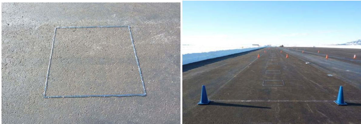
Figure 14 Example of sample boxes (32"x32") laid out on the asphalt surface using silicone sealant in test sections.
