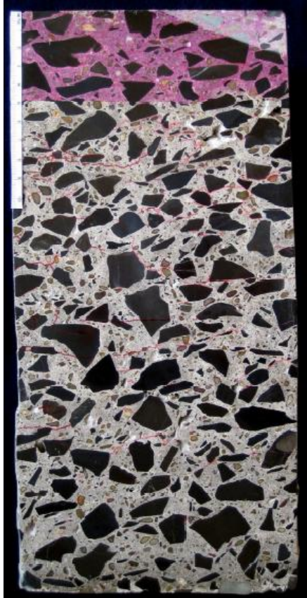
Figure 146: Illustration of the Extent of Microcracking Due to ASR within Core C25MC-D of I80.(ASR Illustrated by Red Lines)
