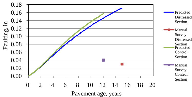
Figure 114: Predicted vs. Observed Joint Faulting for I 79 Segments 470 and 480 (Distressed and Control Sections)
