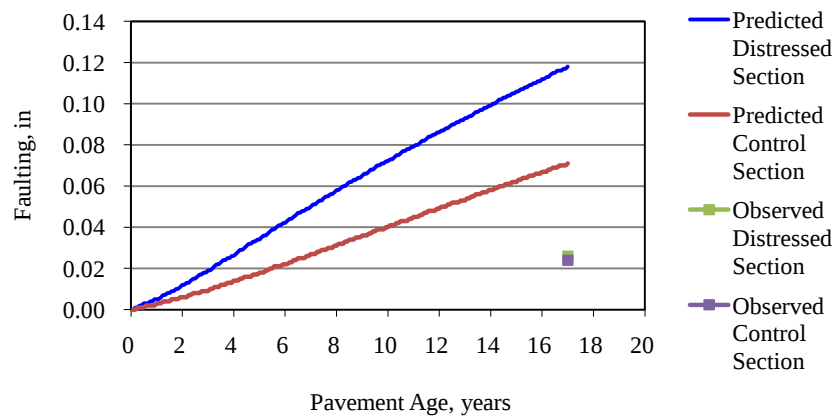
Figure 32: Predicted vs. Observed Joint Faulting for SR 60 Segments 323 and 303 Southbound (Distressed and Control Sections).
