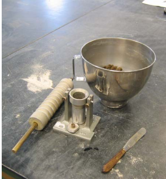
FIGURE 5 PICTURE of the Harvard Miniature Compactor
