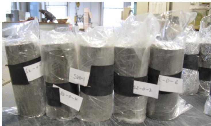
FIGURE 7 Picture of the Soil Specimens Sealed with Sling Film
