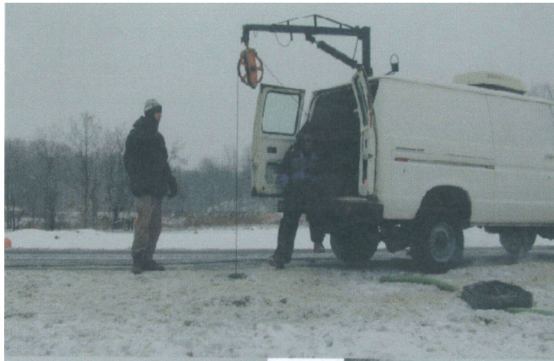
Photograph 7: Set-up for Cross-hole Seismic Shear Wave Measurements
