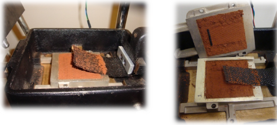
Figure 41. Small-scale pullout tests in Minco silt
