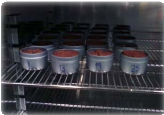
Figure 24. Soil samples in the oven (one sample per bucket) to determine their moisture content
