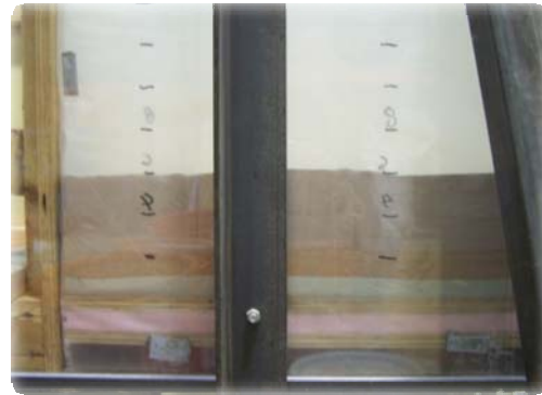
Figure 15. A sideview of the soil and filler panels in the pullout box
