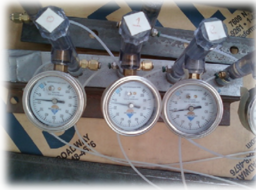
Figure 12. (a) Tensiometer probes placed near the soil-geotextile interface, (b) tensiometer readout dials
