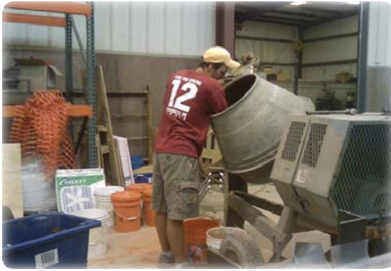
Figure 22. Mixing of Minco silt with water
