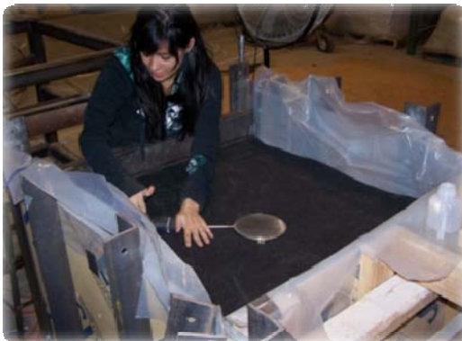
Figure 16. Placement of earth pressure cell on the top of soil in the test box
