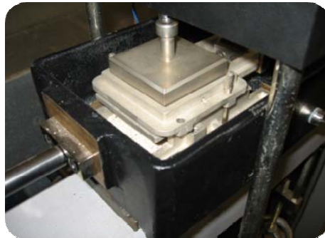
Figure 37. Direct shear test cell
