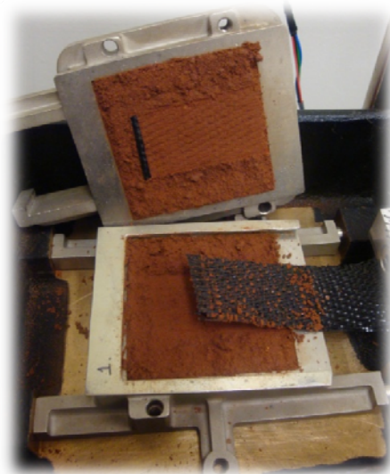
Figure 43. Small-scale pullout test
