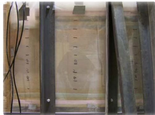
Figure 17. A sideview of the pullout test box filled with soil
