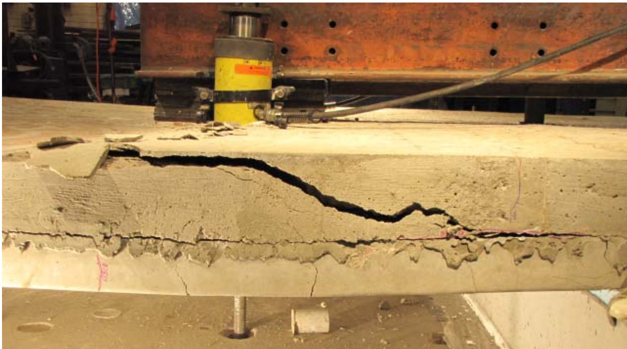
Figure 41: A combination punching shear and sliding failure of Specimen G.
