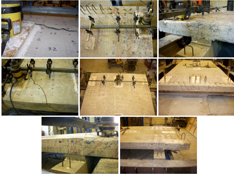
Figure 32: Sample photos for failures after testing.
