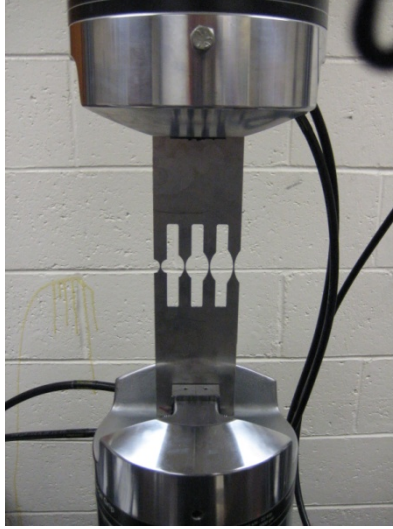
Figure 4: MTS Tensile Fatigue Specimen Test Setup
