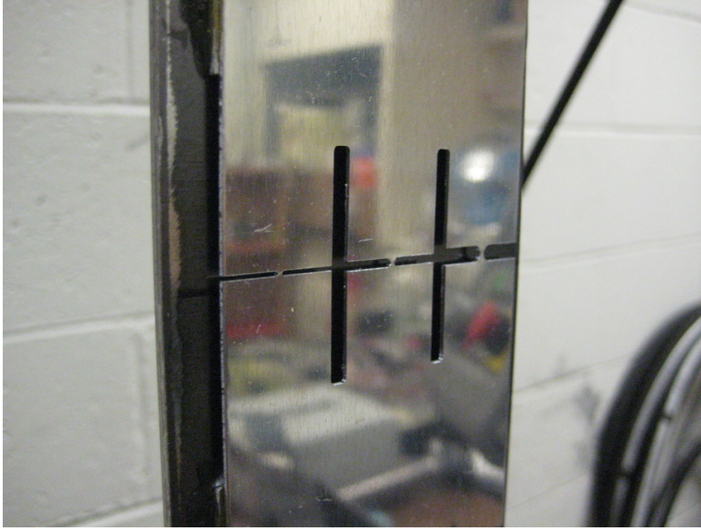
Figure 14: Close Up of Mounted Fatigue Sensor
