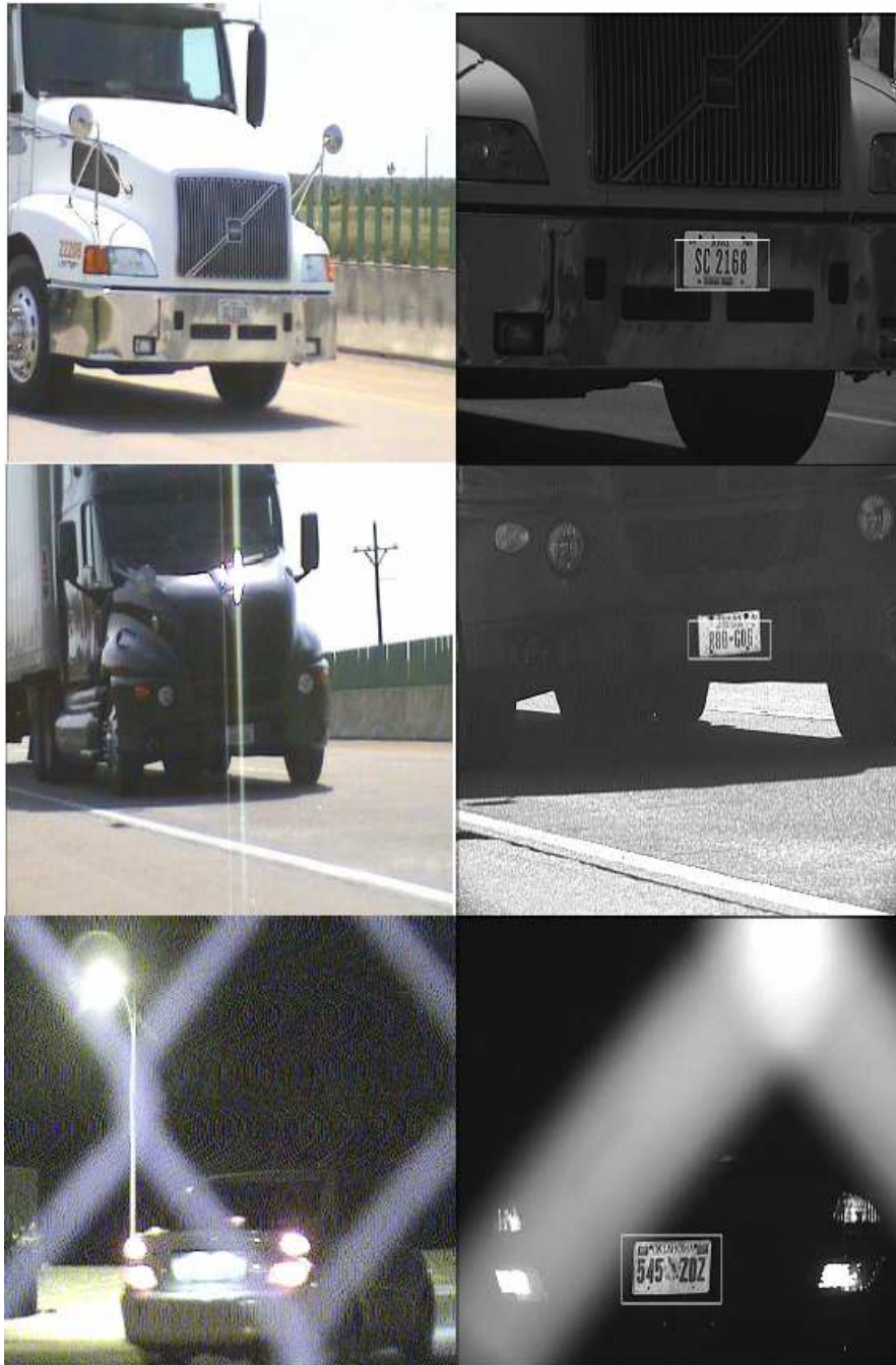
Figure 11. A view of the vehicle cab and license plate is shown in the upper photos for one vehicle and middle photos for another vehicle with lots of sun glare. The Infrared camera technology is very capable of eliminating sun glare to render a usable image. Nighttime images are also possible using the Infrared camera technology as show in lower photos.
