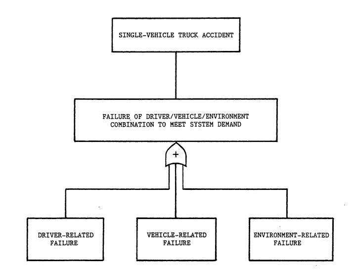
Figure 2. The partial fault tree of a single-vehicle accident.
