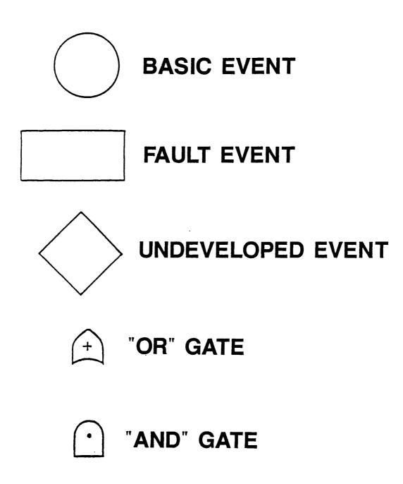
Figure 1. Symbols used in fault tree analysis.
