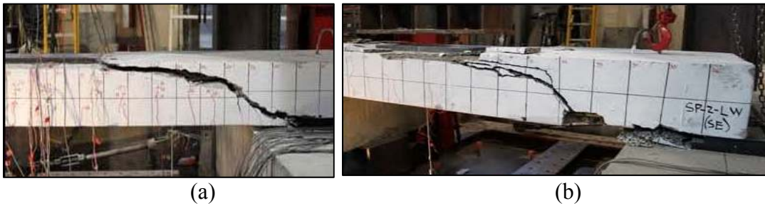
Figure 20. Failure of 2 ft wide panels: (a) NW GFRP panel, (b) LW GFRP panel
