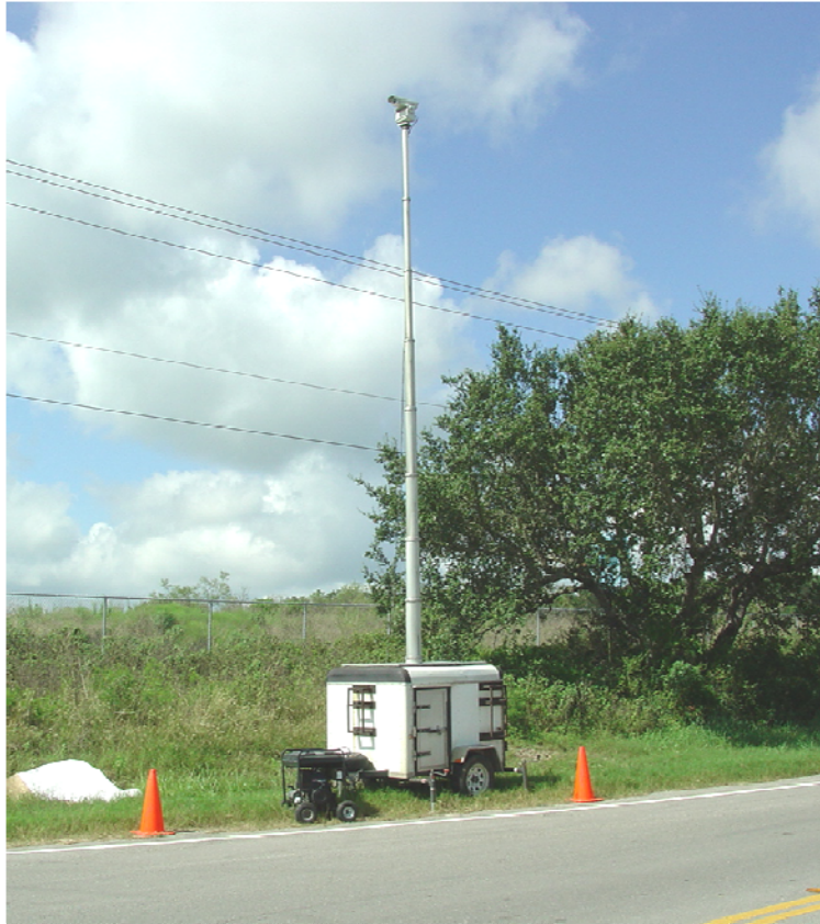
Figure 20. Video Trailer and Telescoping Mast.
