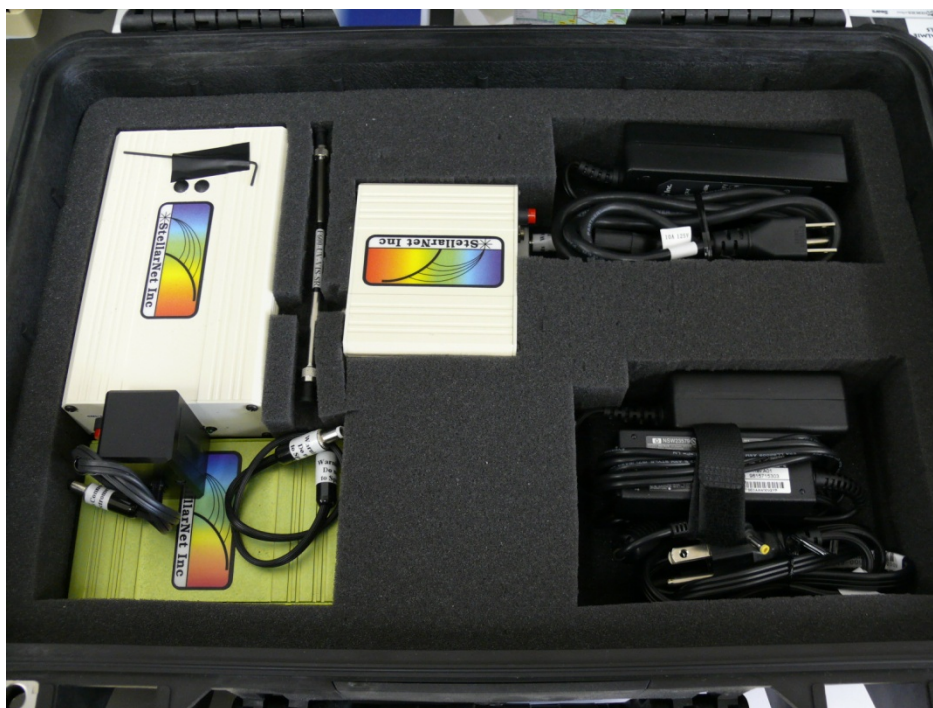
Figure 1.1. Pelican Case with UV-Vis Instrumentation.
