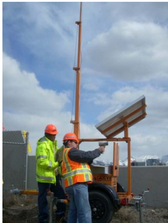
Figure 3-4 Sensor calibration using radar gun (taken by Mitsuru Saito).
