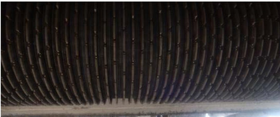
Figure 18. Configuration of taller diamond blades.
