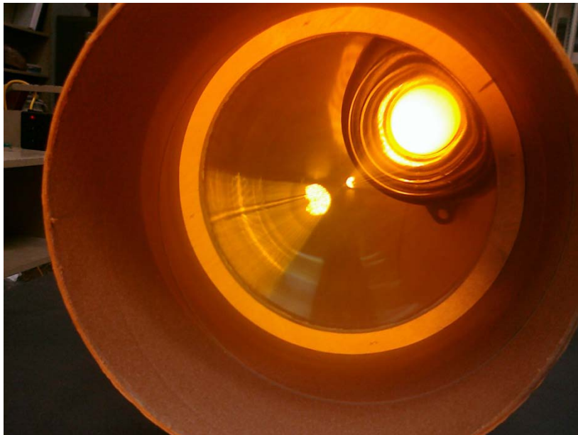
Figure 32. Fresnel Lens Focusing Light From LED Into a Beam Focused on the Light Meter
