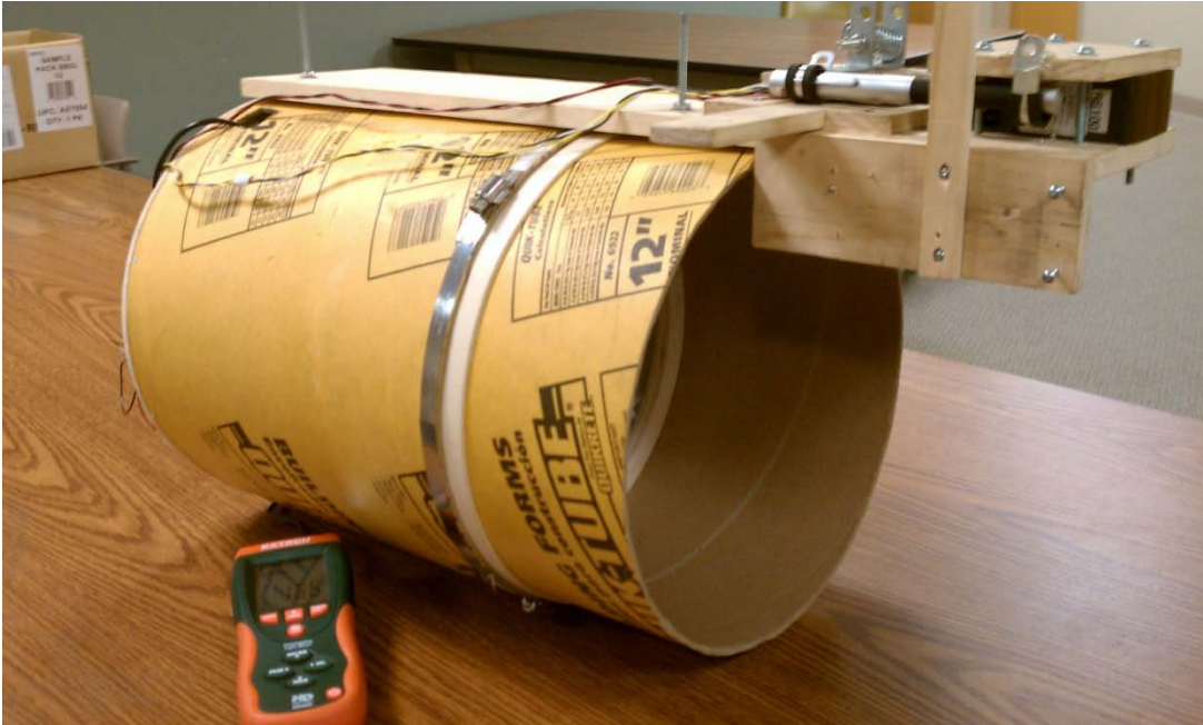
Figure 32. Fresnel Lens Focusing Light From LED Into a Beam Focused on the Light Meter
