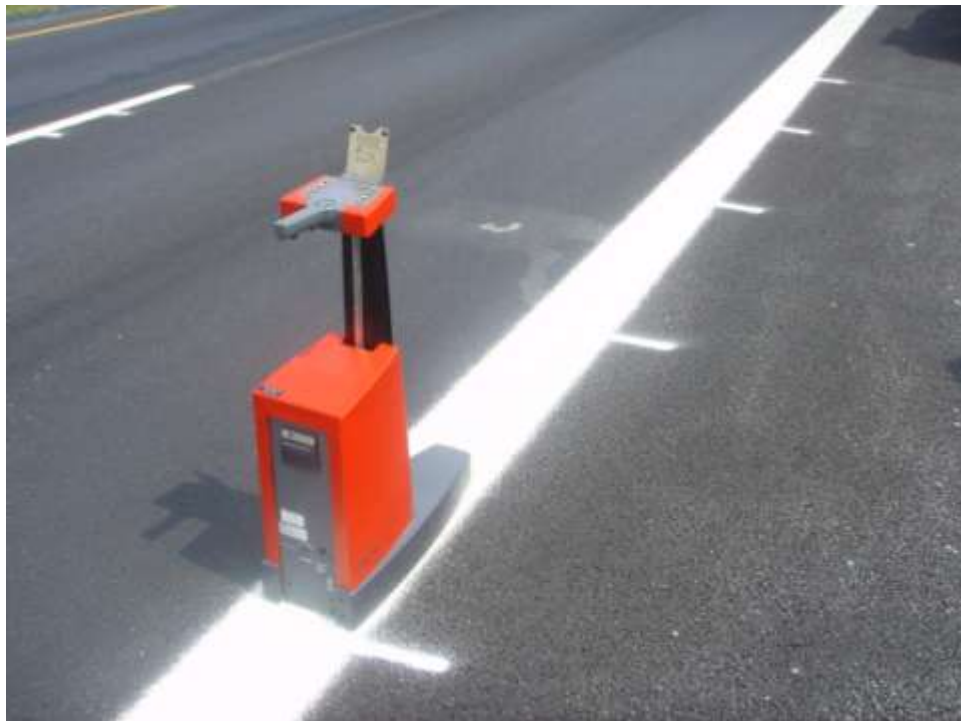
Figure 7. Retroreflectivity Measuring Equipment (Delta LTL-X)
