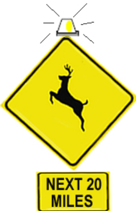
Figure 28. Sign Treatment 2 – Standard Sign with Flashing Beacon.
