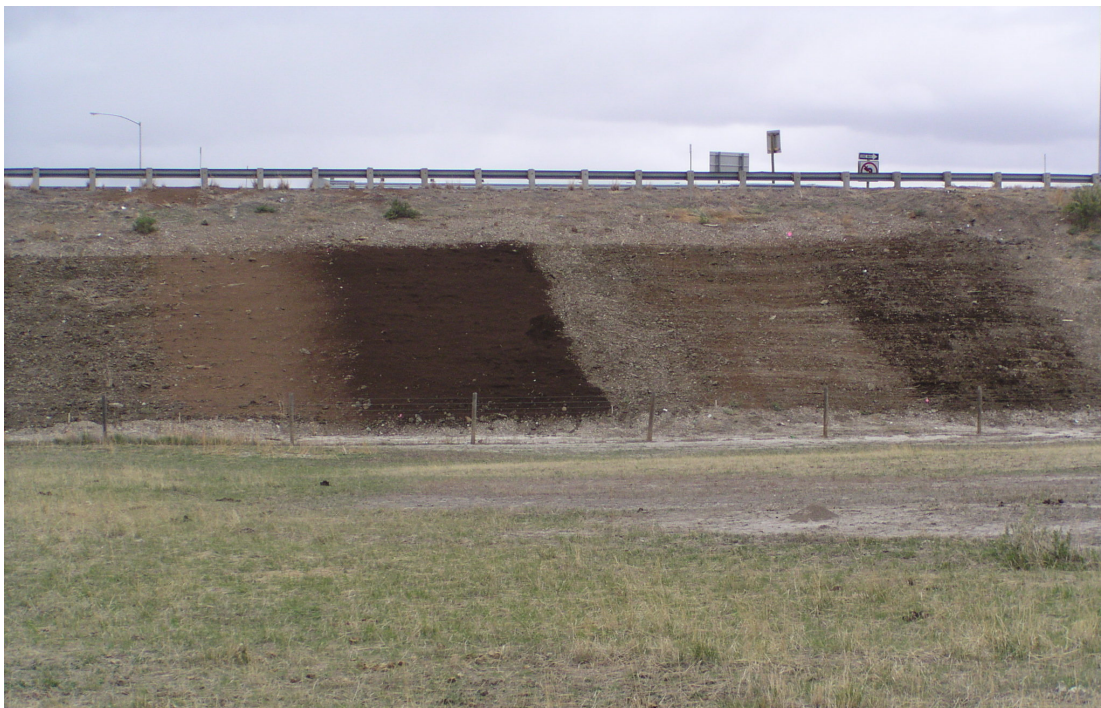
Figure 16. Plots 19 (compost blanket) and 20 (incorporated compost), I-94 off-ramp area, showing Rocky Mountain compost on the left (light-colored) and Earth Systems compost on the right (dark-colored).
