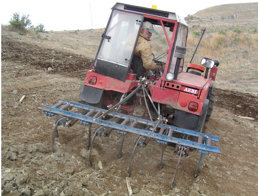
Figure 25. Ford spring-shanked tiller on Plot 20 (Rocky Mountain compost in foreground, Earth Systems material in background).
