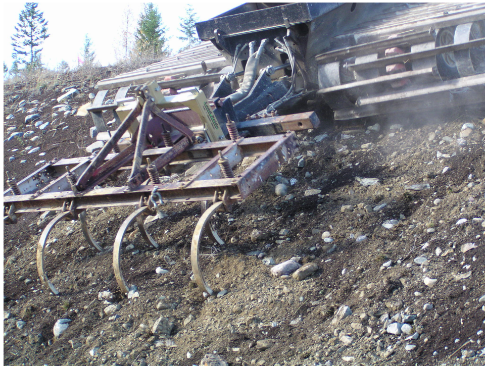
Figure 21. Graham Hoeme 2.4 m (8 ft) spring-shanked chisel plow at the Loon Lake site.
