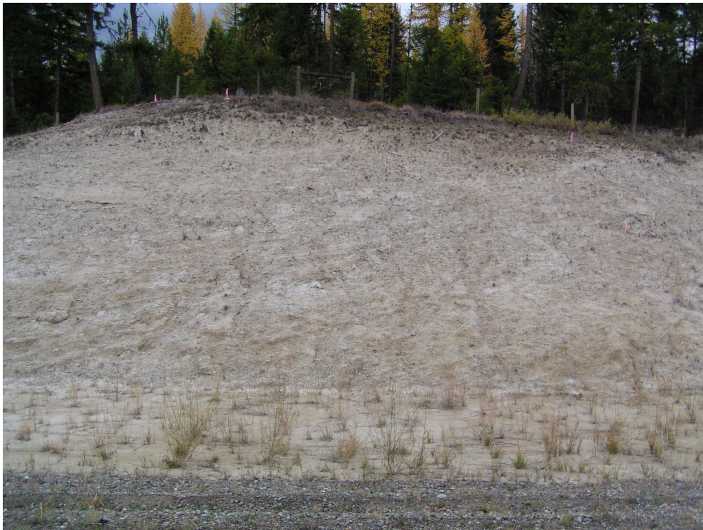
Figure 9. Research Plot 1 at the MP 77 site prior to plot implementation. Note accumulated sediment in ditch, rills and the general lack of vegetation cover.
