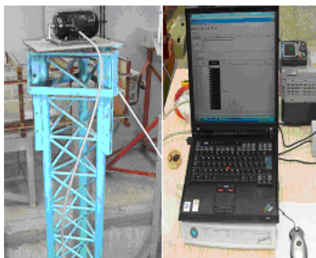
Figure 8 Stand with acquisition system
