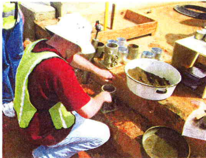
Figure 9. Fabrication of Standard Proctor Sample
