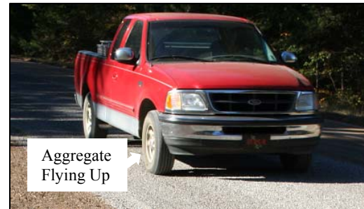
(b) Traffic Prior to Brooming
