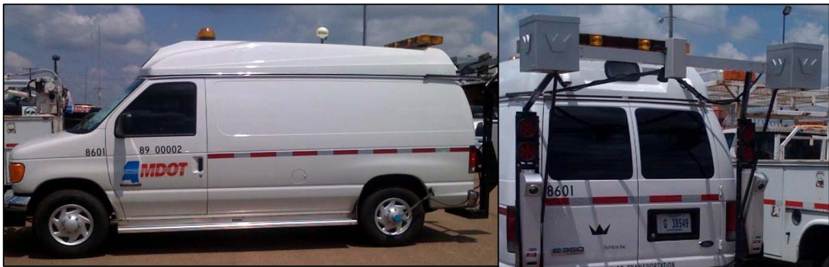
Figure 3.16. Automated Data Collection Vehicle Used for Roadway Profiles
