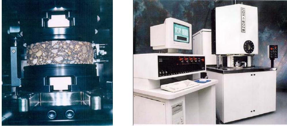
Figure 10 Frequency Sweep at Constant Height (FSCH) test equipment
