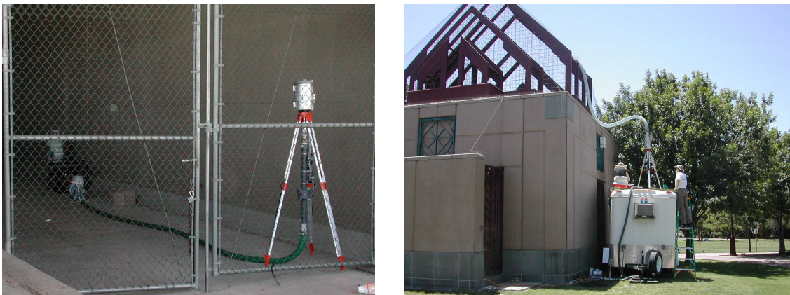
Figure 1: Sampling sites from the May 2004 experiment. Aerosol measurements were made next to entrance of westbound tunnel (left photo) and from the exhaust chimney for the western half of the westbound tunnel (right photo).
