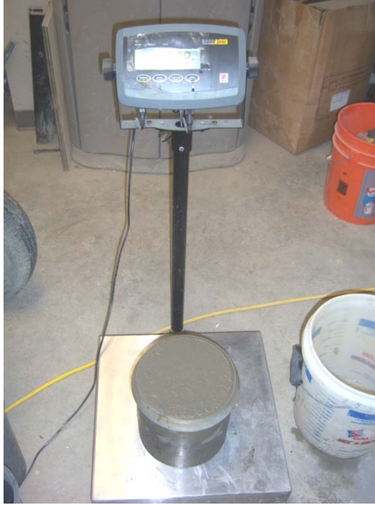
Figure 12: Unit Weight Testing
