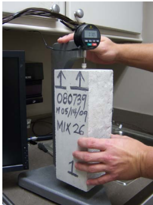
Figure 16: Comparator Reading of Standard Bar
