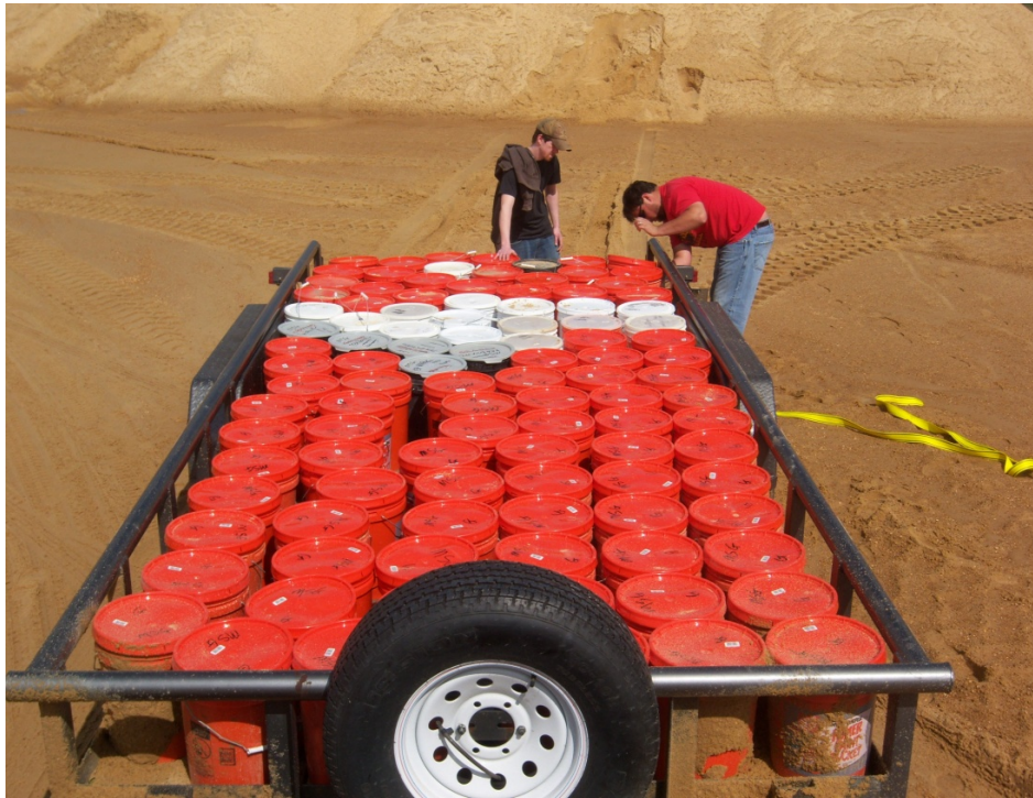
Figure 2: Sampling Gravel Aggregate Source No. 1
