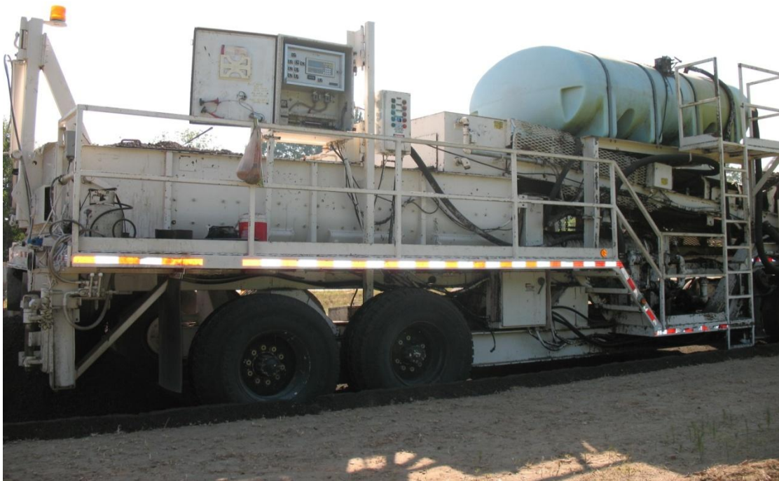
Figure 12: Emulsion Tank and Rate Control Panel
