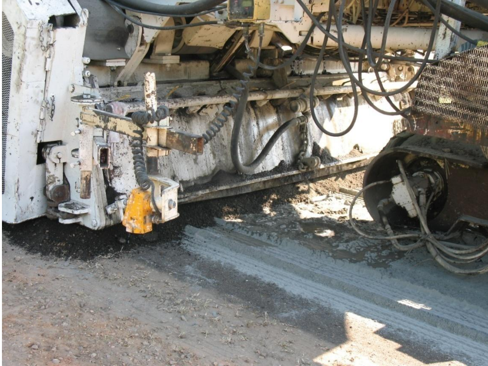
Figure 8: Grinding Head of Reclamation Train
