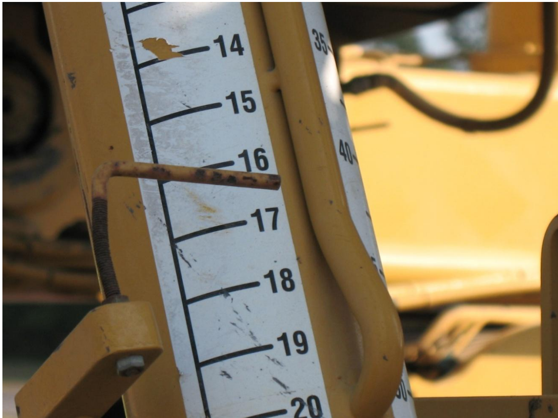
Figure 16: Depth Indicator of RM 500 Mixer
