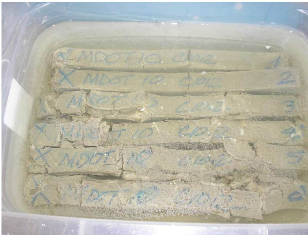
Figure D10. Bars of mortar mix 10 after exposure to sulfate solution for over 1 year according to ASTM C1012.
