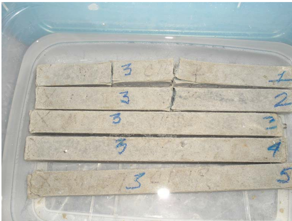
Figure D3. Bars of mortar mix 3 after exposure to sulfate solution for over 1 year according to ASTM C1012.
