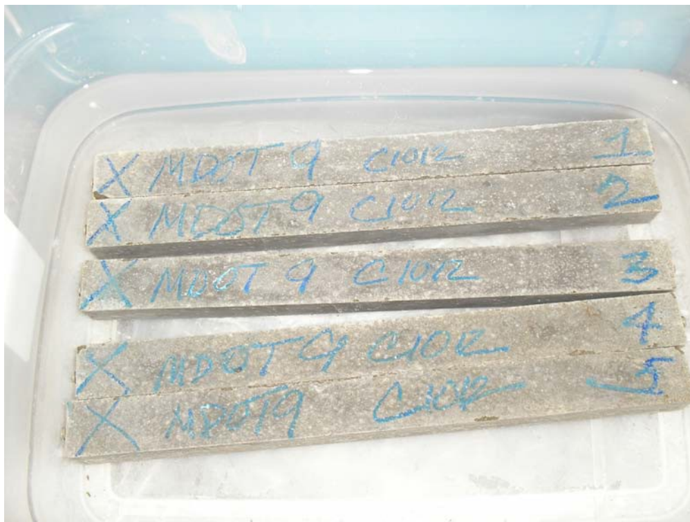
Figure D9. Bars of mortar mix 9 after exposure to sulfate solution for over 1 year according to ASTM C1012.
