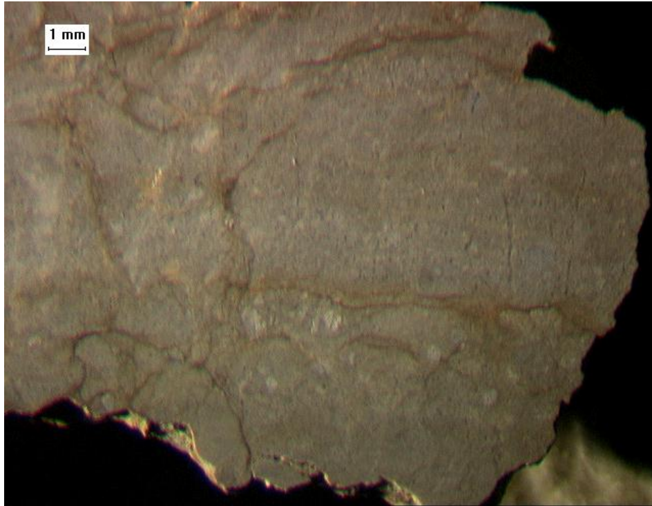
Figure 1. Rockydale aggregate particle showing oxidation along internal boundaries caused by weathering, which weakens the particle
