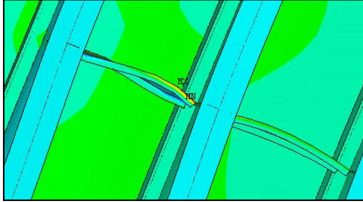
Figure 53. D1-2 and D2-3 with Load at Mid-span, Outer Run
