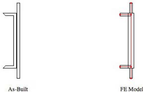
Figure 54. Difference in Field and FE Model Diaphragm-Girder Connections
