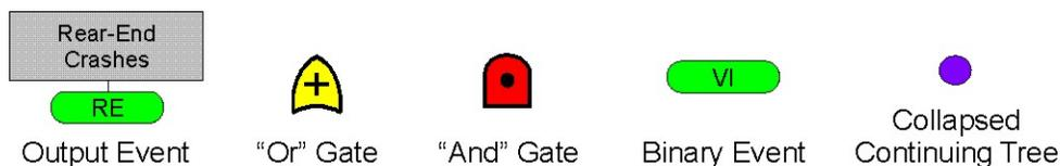
**Figure 3. Symbols Used in Fault Tree Analysis**
