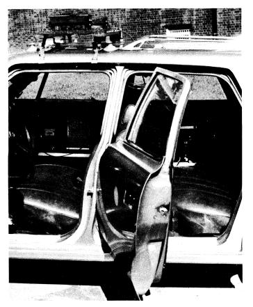
Figure 1. Mobile illumination recording instrumentation with photocells mounted on the roof of the vehicle.
