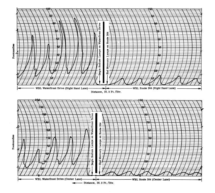
Figure 4. Contrasting illumination levels in the transition area between the mercury lighting on I-264 and the sodium lighting on Waterfront Drive. (Note the difference in the fc. scale factor for the sodium lights in the RHL as opposed to the center lane.)
