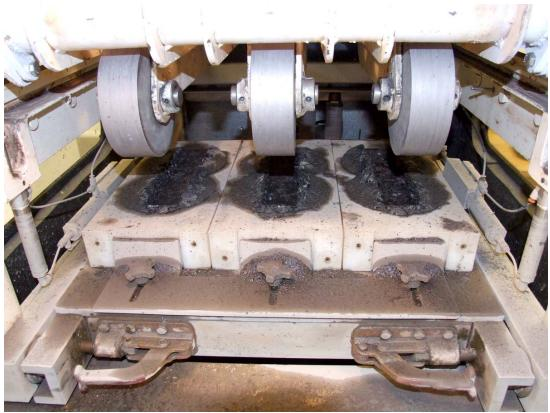
Figure 1. Setup for Hamburg Wheel-Track Test (After Draining)
