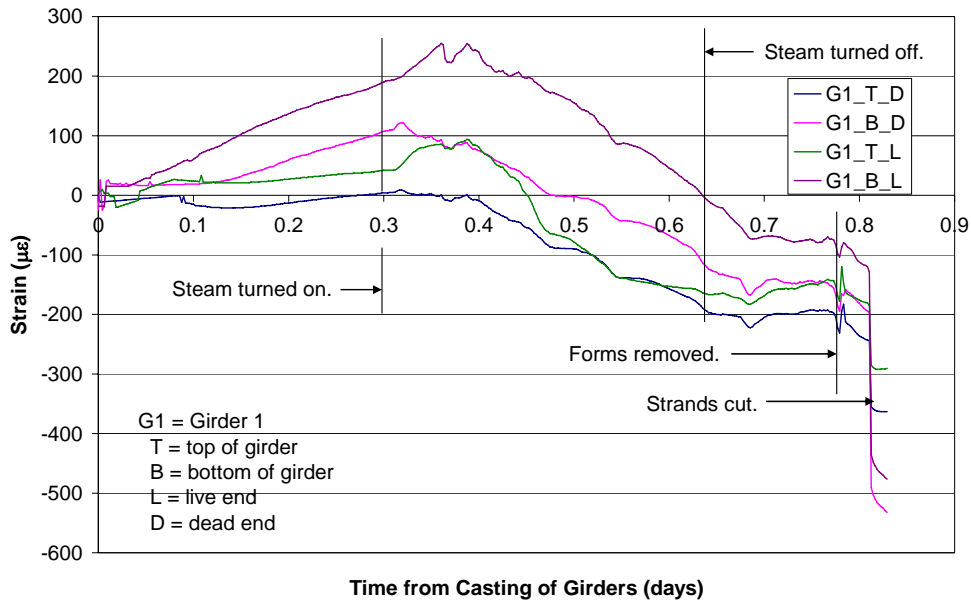
Figure 28. Variation of Strain with Time During Casting and Strand Release for Girder 1.
