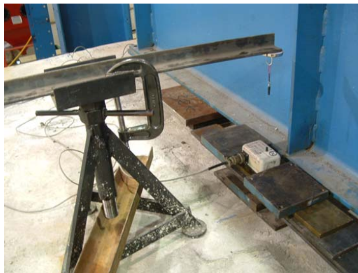
Figure 7. Setup to Measure the Relative Vertical Displacement at the Transverse Joints.
