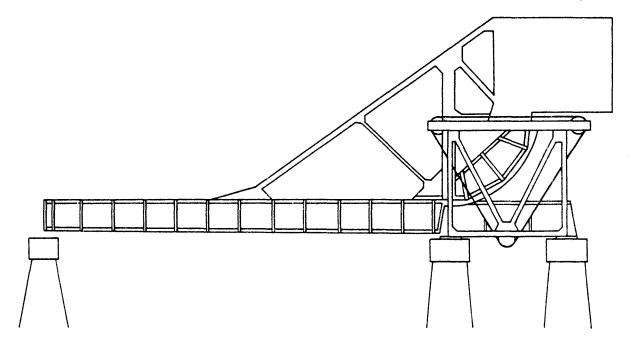
Figure 5. The Scherzer rolling-lift span of the Hodge's Ferry Bridge illustrated in a simple line drawing.
