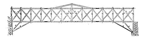
Figure 4. Stephen H. Long's panel truss timber bridge patented in 1830. (From <u>American Building</u>, Carl Condit, illus. 16.)
