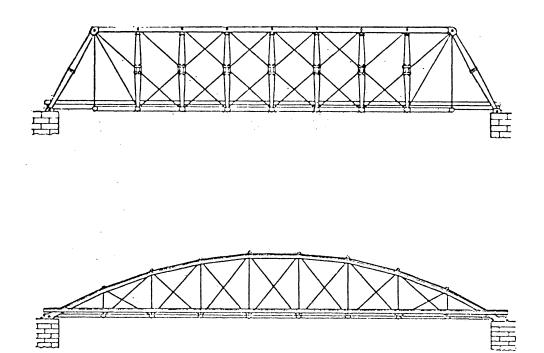
Figures 7 and 8. Squire Whipple's all-iron truss bridges patented in 1847, having cast iron compression members and wrought iron tension members. (From <u>A Span</u> of Bridges, H. J. Hopkins, p. 129.)
