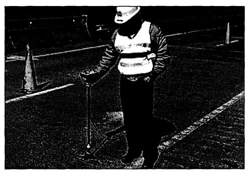
Figure 26. A deck can be marked off into 4- or 5-ft grids, and copper sulfate half-cell potential measurements can be taken at the grid points to identify areas that have a high potential for corrosion (those with measurements more negative than -0.35 volts). Use of a 2-ft grid reduces the chances of missing a high potential area.
