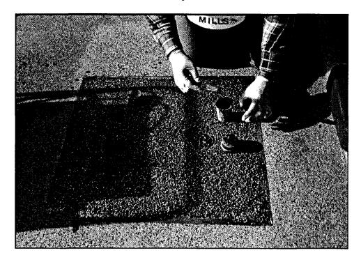
Figure 151. Pipe caps or metal disks required for the tensile bond test should be bonded to the surface of the cored disks with a rapid-curing, paste-like adhesive.
