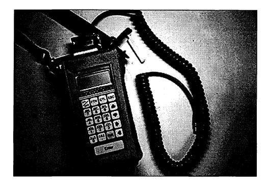
Figure 29. Half-cell potential measurements can be recorded on a datalogger and later downloaded onto a personal computer.
