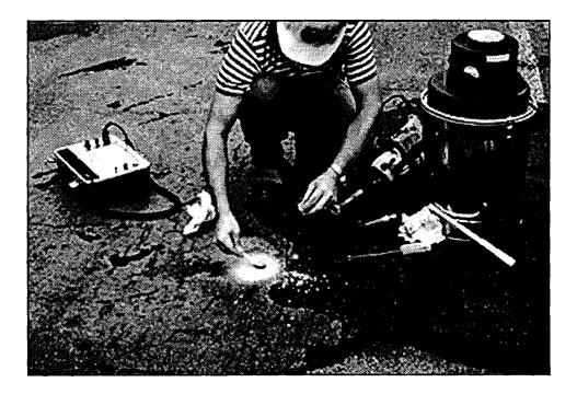
Figure 32. The drill and core barrel should be returned to the hole, and the sample in the vicinity of the reinforcement should be pulverized. A spoon can be used to collect the sample. A chloride content >2 lb/yd<sup>3</sup> can cause corrosion.
