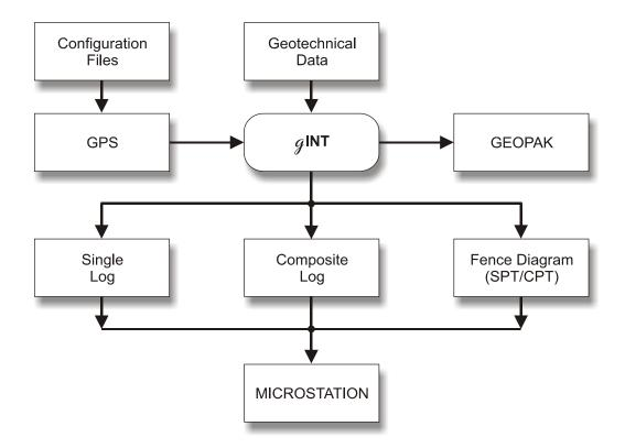
Figure 1. Geotechnical Data Processing at VDOT
