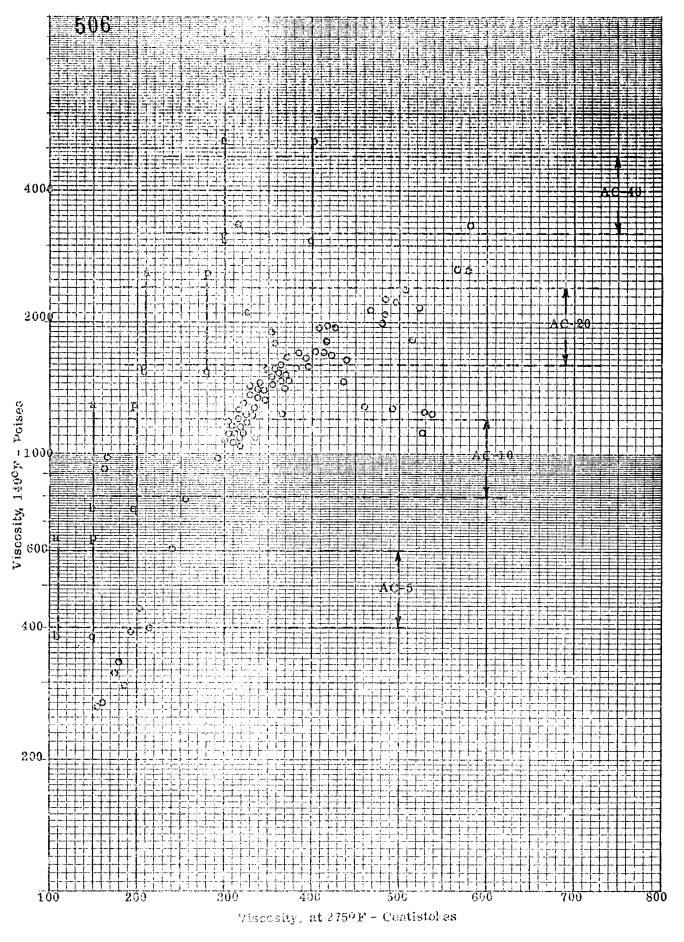
Figure 1. Viscosity at 140°F versus viscosity at 275°F.
