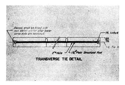
Figure 13. Connection detail requiring field tensioning.
