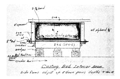
Figure 6. Staunton District casting form for interior beam.
