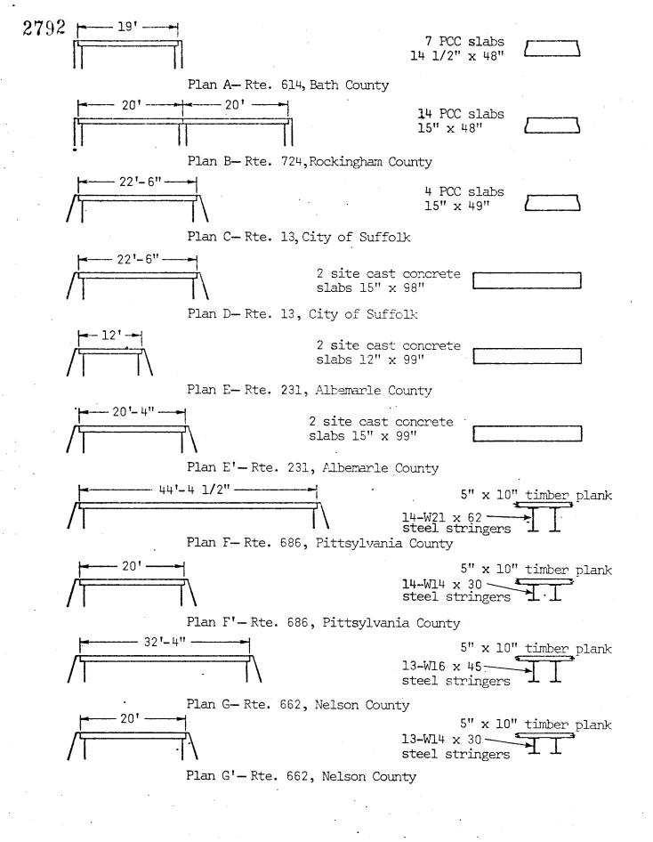
Figure 22. Profile and partial cross section views for bridges considered in quantitative comparisons.
