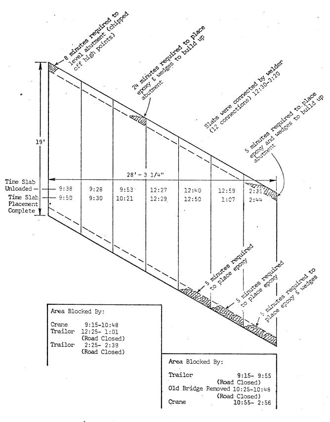
Figure 20. Time and sequence data for Rte. 614 bridge in Bath County.
