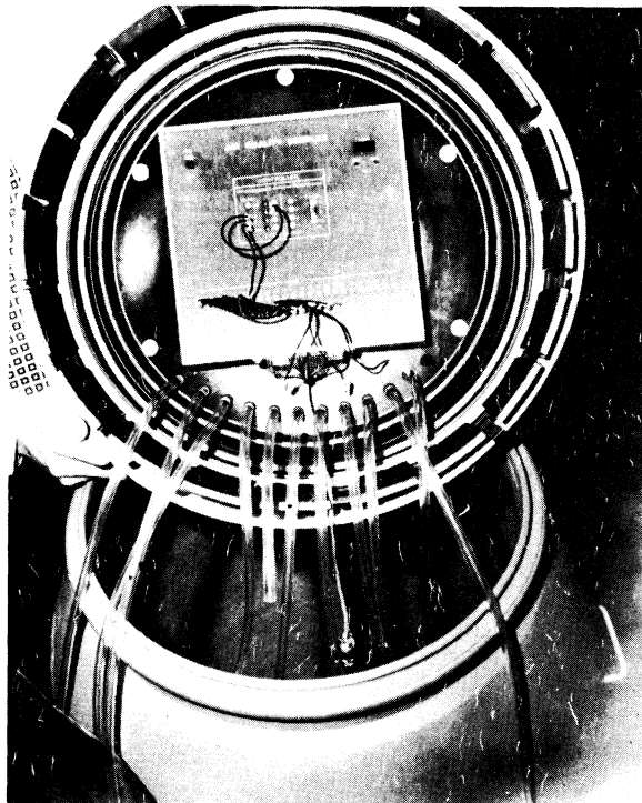
Figure 4. An inside view of the EMI sequential air sampler system. The electronic timing circuit is fastened to the inner side of an unlined cover, which has a hollow chamber where the piston pumps are located (not shown here). Note that this system does not have an inner can to provide neat arrangement of the aluminized nylon bags.
