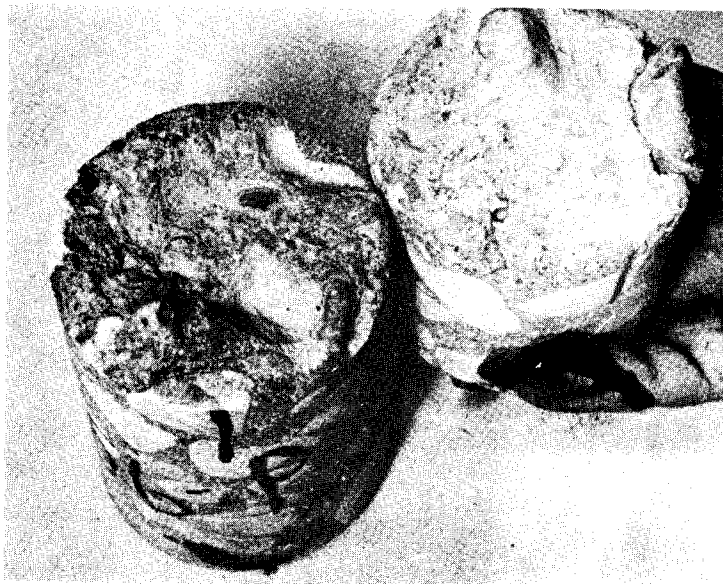
Figure 7. Fracture plane in old pavement containing compacted layer of finely ground concrete underlain by thin coherent layer of calcite.
